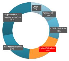
21% of hydrocarbon releases are due to fatigue and high vibration
